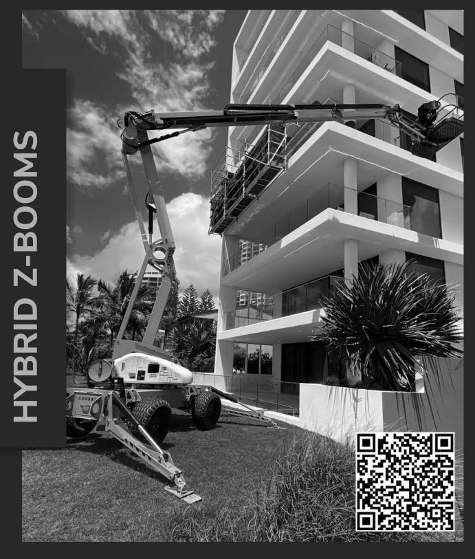
Our Hybrid Boom Lifts range delivers exceptional operating flexibility by combining a small diesel engine with a generator and battery drive This dual-power system ensures efficiency and adaptability across various work environments.
