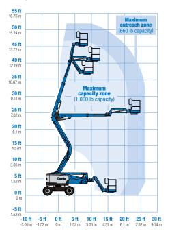
\* The metric equivalent of working height adds 2 m to platform height. U.S. adds 6 ft to platform height. \*\* In lift mode (platform raised), the machine is
