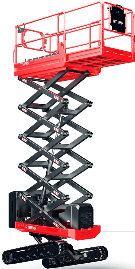
The ATHENA 1090 EVO bi-levelling scissor lift is able to operate on an incline of up to 20° and now can take you to a whopping 10 metre working height.
