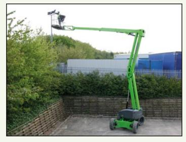
The HR17 Hybrid 4x4 also incorporates ToughCage and SiOPS® technologies. A tough impact resistant composite base and larger cross-section steel give the ToughCage strength and durability, while SiOPS® offers additional operator protection.
